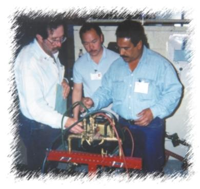
recommendation is a 3.0 psid buffer as this is part of the design criteria. Some of the possible scenarios while testing the reduced pressure principle assembly include the following:
